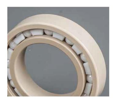
Yes. You can use corrosion resistant plastic bearings dry (unlubricated), which is what we recommend for many applications that expose the bearings to highly concentrated acids and alkalis, or saltwater. This eliminates the problem of lubricant washout in very wet environments. Plastic bearings are only designed for low loads and speeds.
